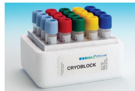
A well-insulated Cryoblock, which can hold up to 20 vials allows operator's to remove a number of vials from the freezer for sub-culture without risk of the culture beads defrosting. The Cryoblock is insulated with a polystyrene shield.
